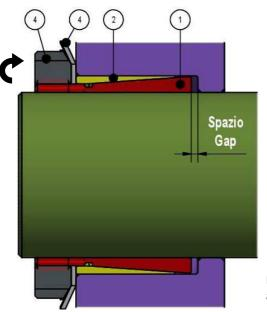
Fig. 4. Positioning of Locking Assembly and tightening of the nut.
