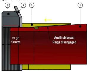
Fig. 3. Disengagement of locking rings.
