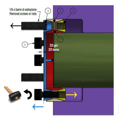
Fig. 4. Release of thrust rings and removal of Locking Assembly.
